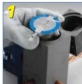
1 Insert CADWELD PLUS package into mould
