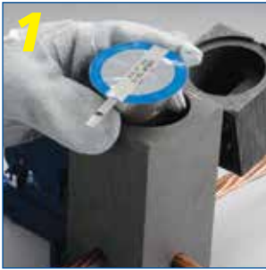
1 Insert CADWELD PLUS package into mould
