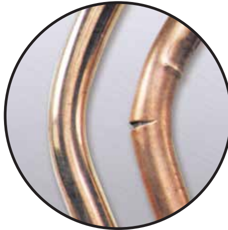
Above photo shows two ground rods subjected to the same pressure load test. The ERICO copper-bonded ground rod, shown on the left, will bend without tears, cracks or folds, to the outer sheath. The inferior copperclad rod shown on the right, has developed cracks and creases to the outer sheath, which will significantly reduce its serviceable life and put the integrity of the entire electrode at risk.
